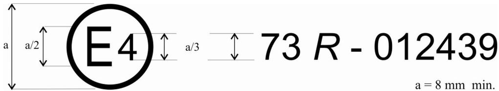
The above approval mark affixed to an LPD shows that the LPD type concerned has, with regard to its lateral protection, been approved in the Netherlands (E 4) pursuant to Regulation No. 73 under approval number 012439. The first two digits of the approval number indicate that the approval was granted in accordance with the requirements of Regulation No. 73 as amended by the 01 series of amendments.
