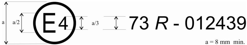
The above approval mark affixed to a vehicle or to an LPD shows that the vehicle type concerned has, with regard to its lateral protection, been approved in the Netherlands (E 4) pursuant to Regulation No. 73 under approval number 012439 as a complete vehicle. The first two digits of the approval number indicate that the approval was granted in accordance with the requirements of Regulation No. 73 as amended by the 01 series of amendments.
